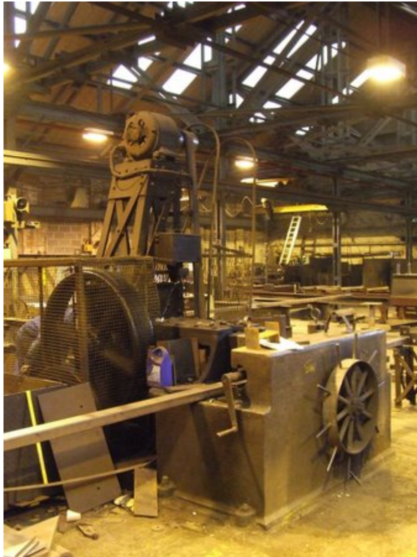
Above – Photo of the historic bending machine in Leonard Cooper’s Balm Road works (photo Derek Rayner)
